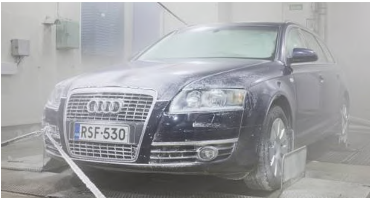
Figure 5. Testing of cold properties with diesel cars in a climate chamber.
